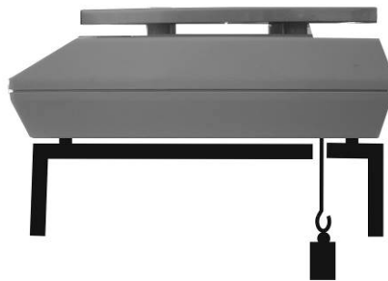
Fig. 1: Setup of balance for underfloor weighing
