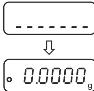
**i** In case of the adjustment error (e.g. object on the plate) the following error message will be displayed: <CAL NO>, repeat the adjustment procedure.
