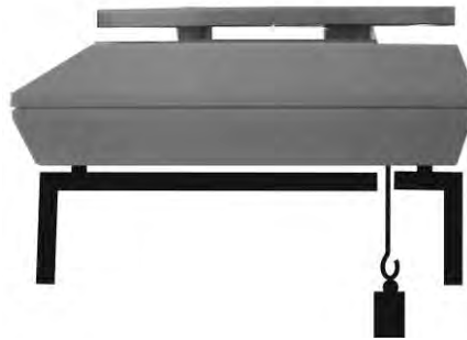
Fig. 1: Setup of balance for underfloor weighing
