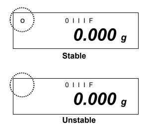
The balance is in a stable condition if the [o] stability indication appears on the display. The [o] indication disappears if the condition is unstable. Stable ambient conditions can be achieved by using the draft shield (See chap. 5.2.4 for installation)
