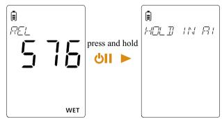
A scrolling text appears mentioning "hold in air and press right" hold the unit in air, away from any other object and then press key to calibrate the device for REL mode.
