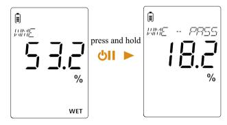
press >> key to exit the calibration check.
