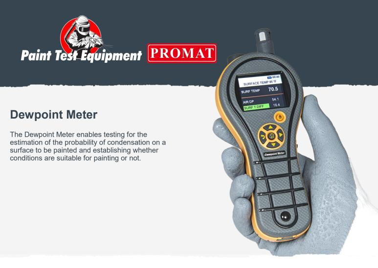
The steel surface temperature generally should be at least 3°C above the dew point when paints are applied. Below this temperature the Dewpoint Meter will sound an alarm and the display colour will change to warn you that the surface conditions are not suitable too paint.
