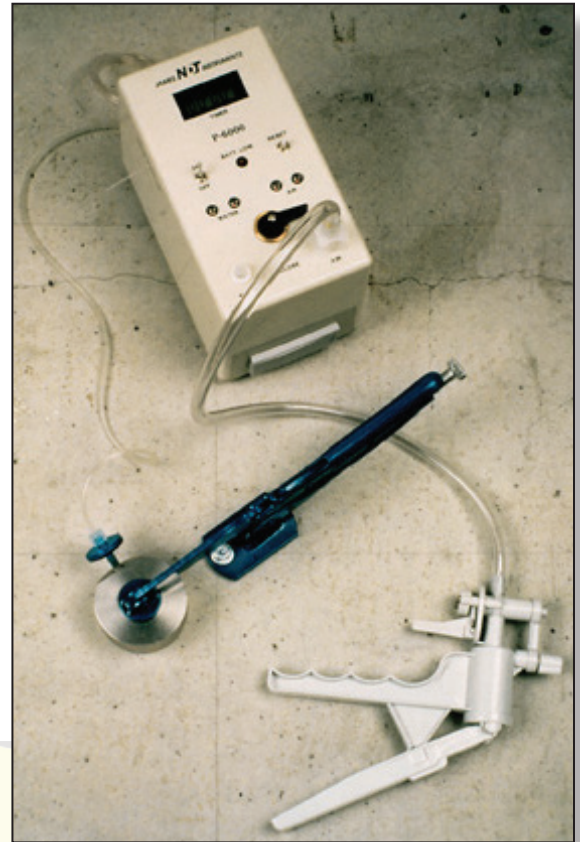
Surface Permeability Test
