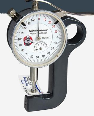
The Replica Tape Gauge is used to measure the Testex Replica Tape replica and determine the average maximum peak-to-valley height of the blasted profile.
